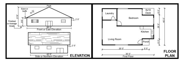
Building elevation drawings are exterior views of the building, sometimes identified as front, rear, left or right or North, South, East or West. Elevation drawings must be:
